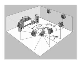
Arrange the speakers around the center of the room based on the angles shown in the illustration on the left. If you are unable to position the speakers according to the angles shown, place one set of surround speakers slightly forward of the listening position (toward the front speakers).
